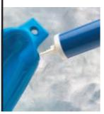
Remove screw from casing. Insert Polyform hand pump.
