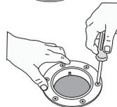
Install using only a HAND-HELD screwdriver. DO NOT over-tighten the screws.
