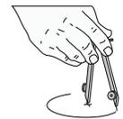
Carefully choose the location on deck where the cowl vent will be installed. If a hole saw is to be used, mark the center of the installation spot with an "X" for the pilot bit to penetrate. If a saber saw is to be used, scribe the circumference of the hole with a compass. A 3" deck plate requires a 3-3/4" (95mm) hole and a 4" deck plate requires a 4-3/4" (121mm) hole. Do not use the
