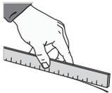
Check the camber of the deck by placing a 12" (300mm) straight edge on the deck installation location and rock it. Rotate the straight edge 90 degrees and repeat. Do not install the deck plate in an area with more than 1/2" (12mm) of camber over 12" (300mm) length of deck surface. Too much camber will distort the vent's deck plate and may result in water leakage.
